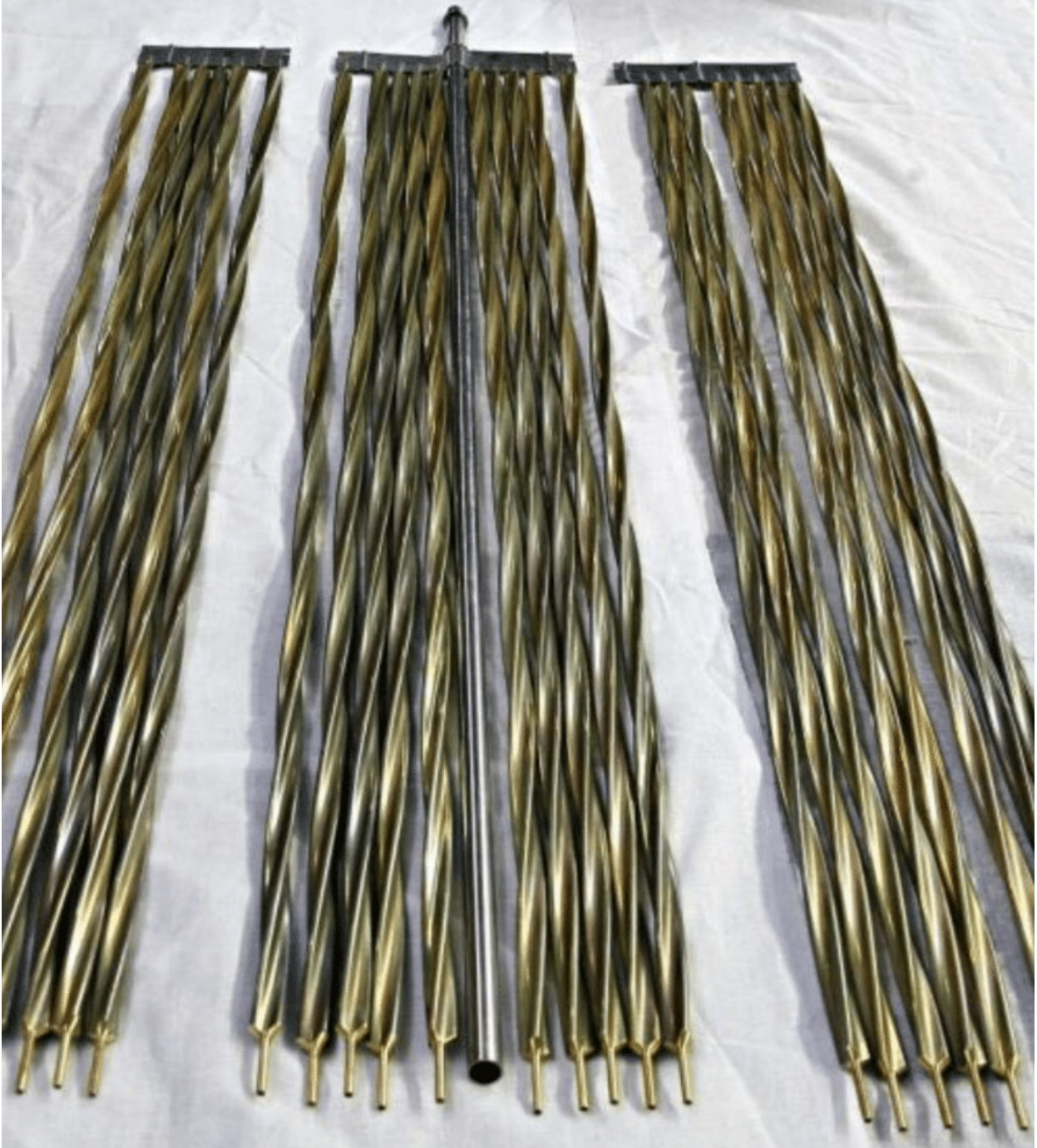
Mock-Up of Four-Lobed Helical Fuel Rods.
